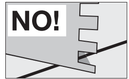
NEVER bang a trowel or other tool on the heating cable.
